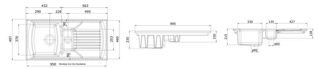
NB: Due to manufacturing processes this sink may have a +/- 3mm tolerance on the measurements.
