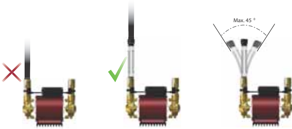
Fig. 18 Connecting the flexible hoses
