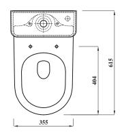
**Special notes** Pan fixes to floor using side fixing bracket supplied with pan.
