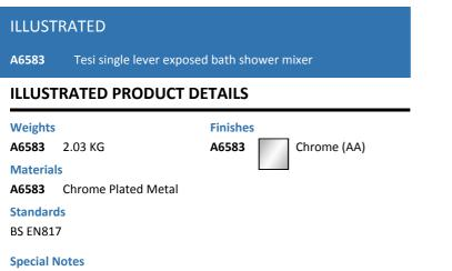
Suitable for balanced supplies. Consideration should be given to safe hot water delivery and the use of an appropriate temperature reduction device, please see A5900AA (for use with 15mm pipework) or A5901AA (for use with 22mm pipework). Unregulated flow rate 15 litres per minute at 1.5 bar and 21 litres per minute at 3 bar.
