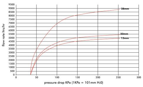
these values are obtained with: Inlet pressure 8 bar and outlet pressure 3 bar
