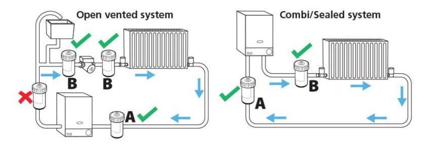
In both diagrams, position **A** is recommended as part of ADEY's Best Practice<sup>™</sup> approach. Position **B** is suitable if space is tight on the return.
